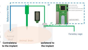
Attach a distinct wire as a Ground Wire to the ground hole on the top of the probe connector or the bottom of the headstage. Connect this wire to the bone screw anywhere on the animal skull.
