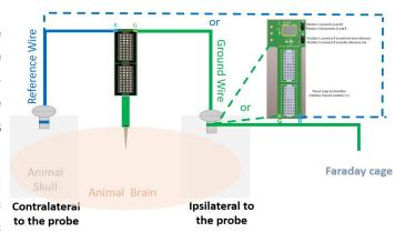
These wiring configurations will aid in establishing proper reference and grounding connections for your 64-channel acute electrode setup.
